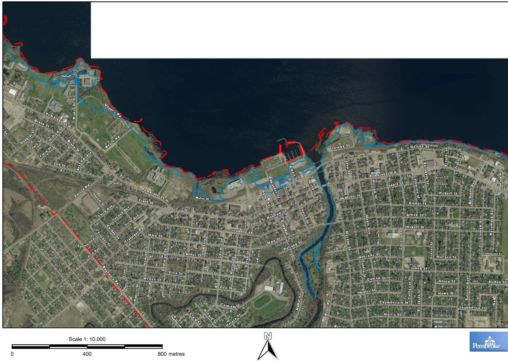
Figure 2-2: Ottawa River Floodlines (in blue) within the Study Area (dashed red lines) for the 100-year Flow Event
