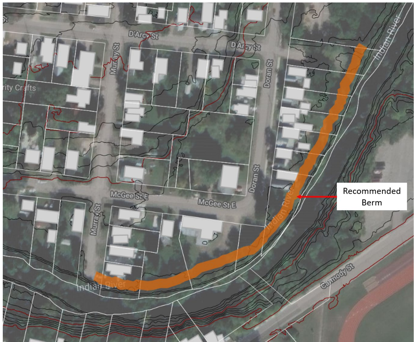
Figure 4-6: Extent of the Recommended Berm
